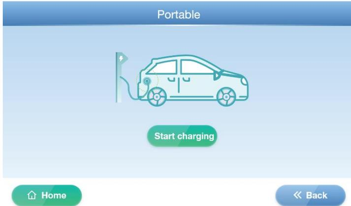
Click the Start charging button, the charger will automatically detect for a few seconds and start charging. The charging interface displays Battery SOC, Charging time, Battery type, Charging voltage, while Portable charging does not display Card Balance, Charging current, Amount charged, or Cost information.
