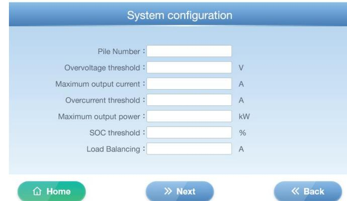
2) Click the Next button to navigate to the second page of System configuration, where you can view and modify relevant parameters:
